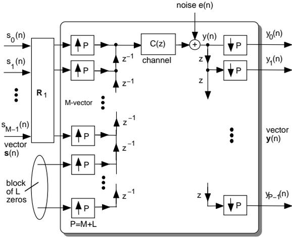
**Fig. 3.** The zero padding system with precoder  $\mathbf{R}_1$ .
