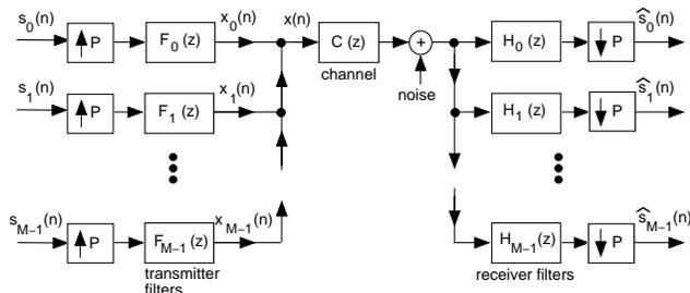
Fig. 1. The transmultiplexer system ( $P \geq M$ ).
