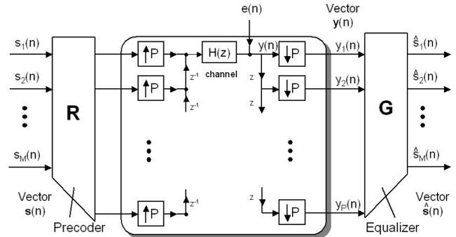
Fig. 1. Communication System with Redundant Filter Bank Precoders
