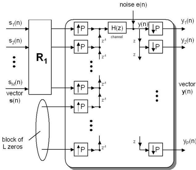
Fig. 2. The zero-padding system with precoder  $\mathbf{R}_1$
