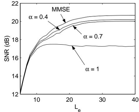
Fig. 3. Overall SNR as a function of equalizer length.
