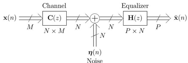
Fig. 1. MIMO channel-equalizer model.
