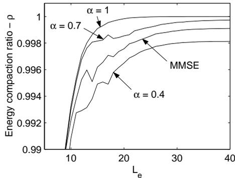
Fig. 2. Energy compaction as a function of equalizer length.
