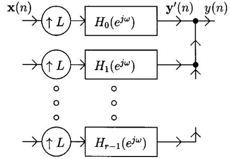
Fig. 11. Synthesis filter bank—a special case of Fig. 10.
