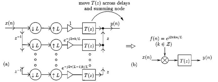
Fig. 18. Illustrating the proof of Theorem 2. (a) Rational LPTV( $L$ ) system producing WSS output for all WSS inputs. (b) Equivalent structure for this system.
