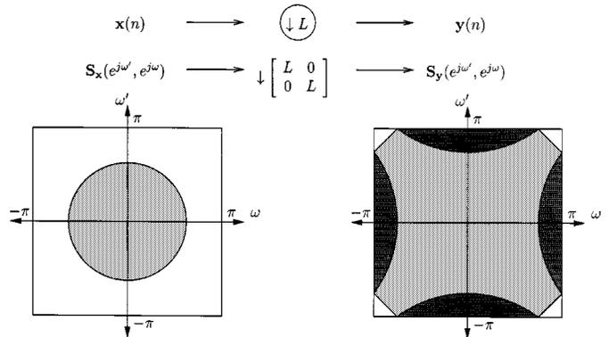
Fig. 9. Effect of a decimator on the bispectrum of a nonstationary process.
