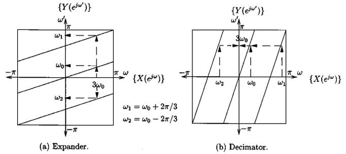
Fig. 4. Bifrequency maps of three-fold expander and decimator. (a) Expander. (b) Decimator.
