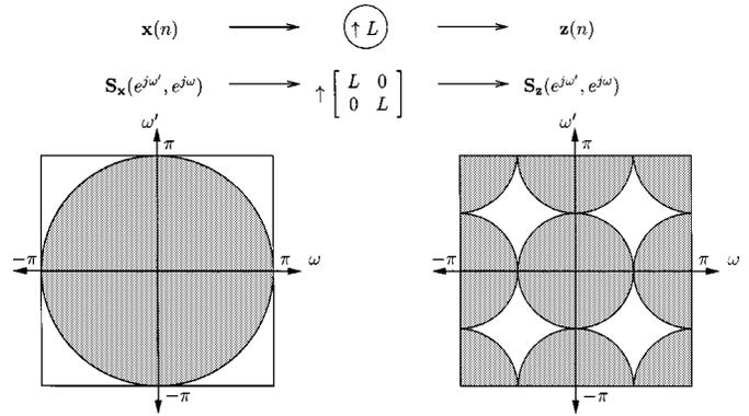
Fig. 8. Effect of an expander on the bispectrum of a nonstationary process.
